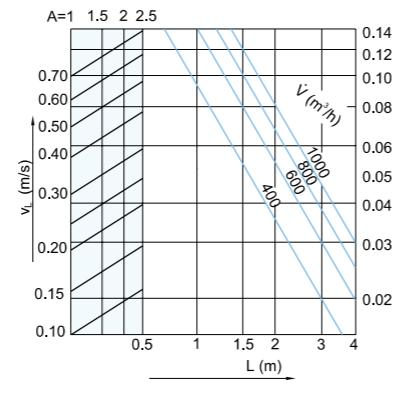
Diagrams of mean jet velocity  $v_h$  at distance B and diagrams of mean jet velocity along the wall  $v_L$  and temperature ratio for diffuser DEU (600 - 800)
