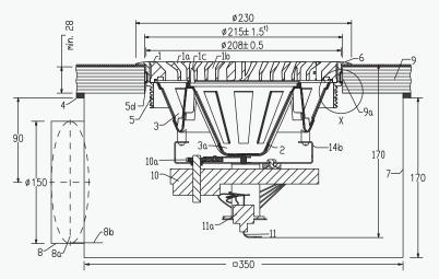
ISF-AD with RR mounting ring, optional electric VAV actuator, and optional connection box type  $\mathsf{CK}$
