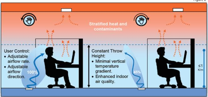
Damper stops offer a choice of fixed airflow rates and adjustable airflow rate ranges, including ones of marginal adjustability (table 1). User-adjustable airflow rate throttling may be marginal or eliminated entirely, if desired, due to the availability of discharge direction adjustment as an alternative to achieve thermal comfort personalisation by the user. This enhances indoor air quality by maximising airflow rates.
