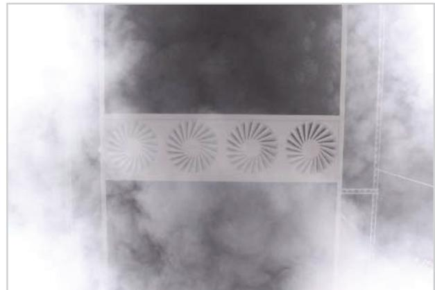
Figure 1: Smoke pattern at maximum airflow
